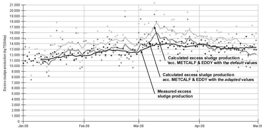
**Figure 3:** Observed and calculated sludge production at the investigated sewage treatment plant according to METCALF & EDDY. The calculations have been carried out with the default and the adapted values from Table 2.
