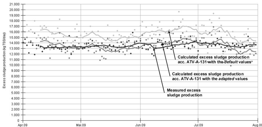
**Figure 2:** Observed and calculated sludge production at the investigated sewage treatment plant according to ATV-A-131. The calculations have been carried out with the default and the adapted values from Table 2.
