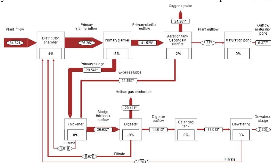
**Figure 1:** COD mass balance of the investigated sewage treatment plant. The listed flows are in kg COD/day. Values inside the boxes represent the balance results in % (eDAB® full plant view).
