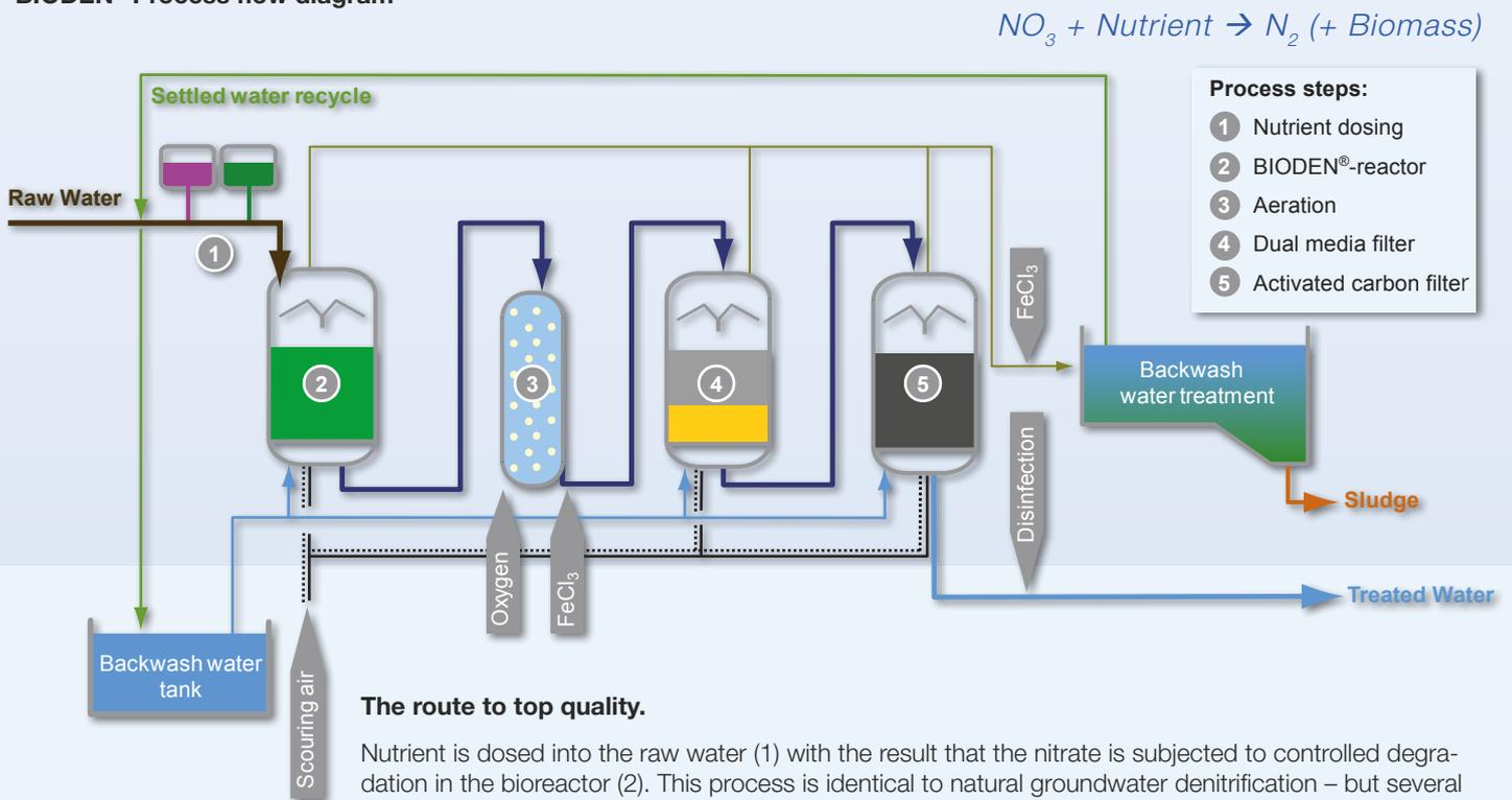
Nutrient is dosed into the raw water (1) with the result that the nitrate is subjected to controlled degradation in the bioreactor (2). This process is identical to natural groundwater denitrification – but several times faster. Subsequently, the water is enriched with oxygen (3) and subjected to post-cleaning by means of flock and activated carbon filtration (4,5). Finally, the water is disinfected by e.g. UV radiation.
