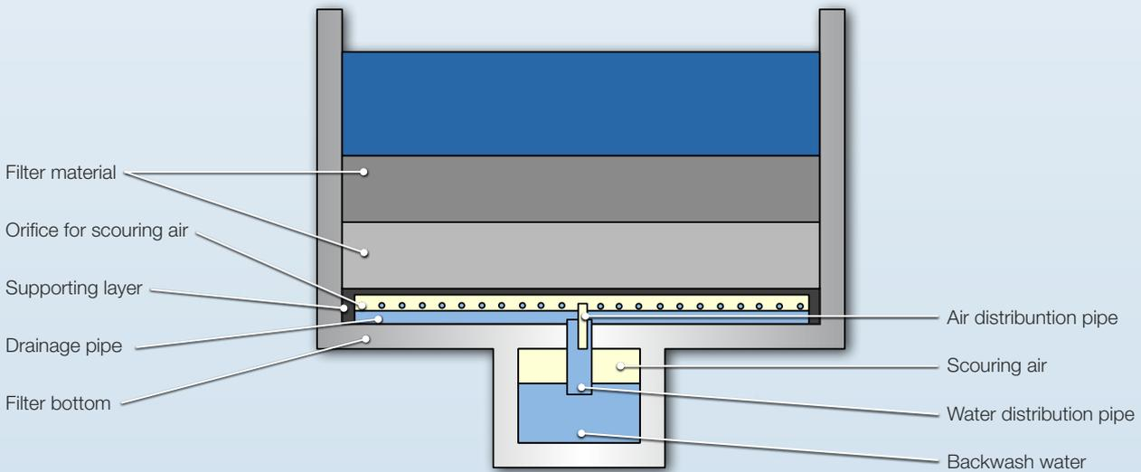
Sludge water extraction is based on the gradual opening of the flap valve, which prevents filter media loss, even where this is highly possible as in the case of specifically light media. This allows an additional degree of flexibility with regard to filter media combinations.
