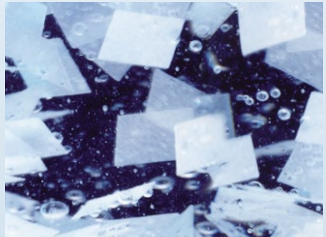
FLUOPUR® carrier material in the moving bed
