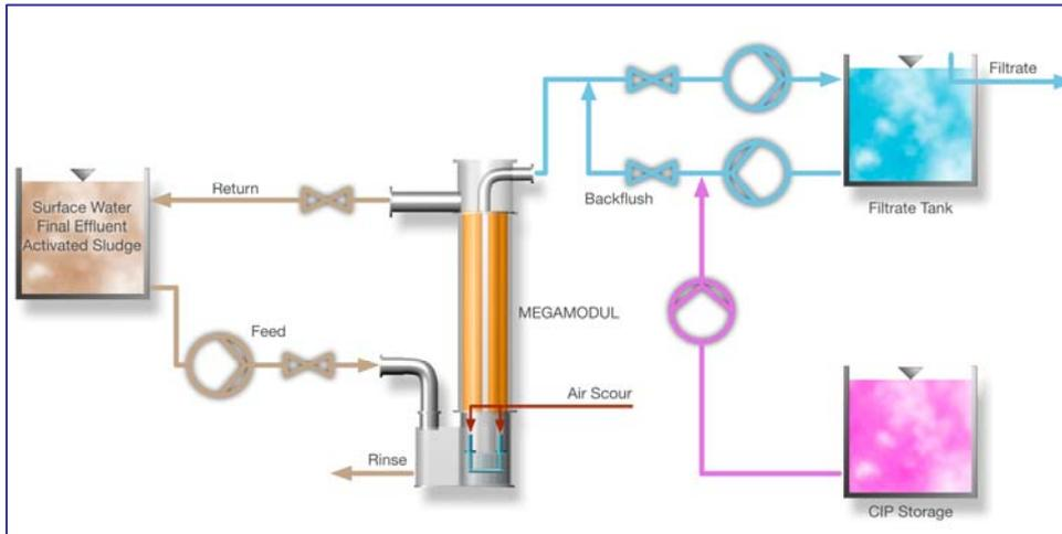
**Figure 4.1** MARAPUR process with the MEGAMODUL
