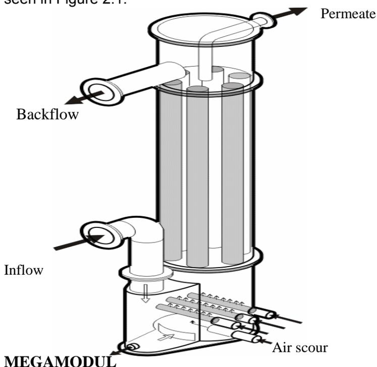
**Figure 2.1** Main design features of the MEGAMODUL
