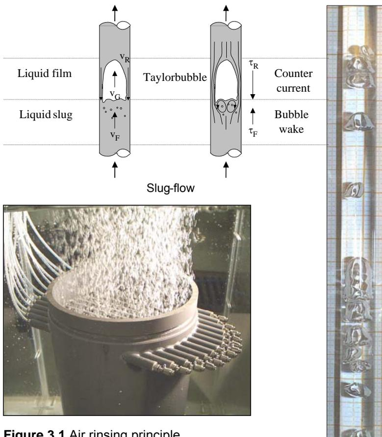
**Figure 3.1** Air rinsing principle
