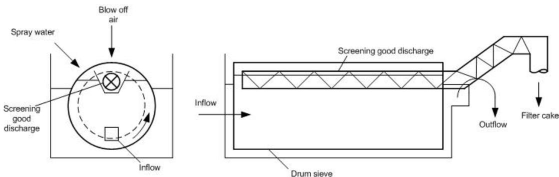
**Figure 5.1** Fine sieve for MEGAMODUL pretreatment
